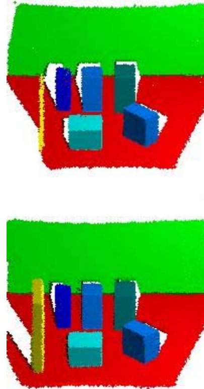
Figure 4. Rendered image from voxel array after initial sensor image, and after the accumulation of 10 images (2 nd ). Note the new portions of the scene encountered after all 10 images are accumulated. Also note the reduction in the missing data (white areas).
